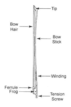
Your bow is made up of several different parts. Some of the parts move and some are fixed in place.
