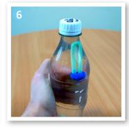
Screw the lid onto the bottle and tighten. Firmly squeeze the sides of the bottle, hold, and then release. The 'submarine' should sink with each squeeze and surface with each release.
